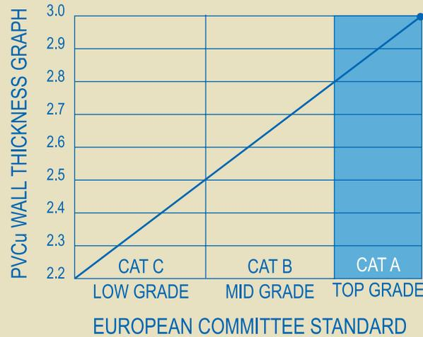
All Ultimate main frame walls are 3mm thick which offers incredible frame strength and rigidity that will last for years.
